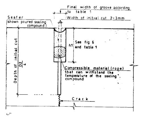
43 – 3 Construction Joint - Detail A
