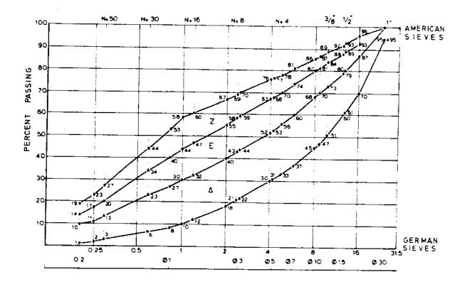
DIAGRAM 1: GRADING LIMITS FOR AGGREGATES OF MAXIMUM GRAIN PASSING Ø 30, or # 31.5, or 1"
