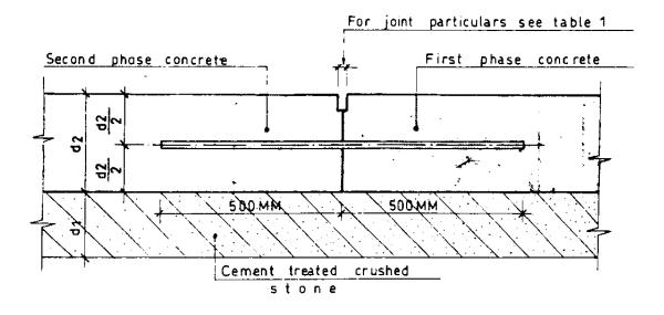
Fig. 43-5a : Longitudinal Joint provided with anchoring bars
