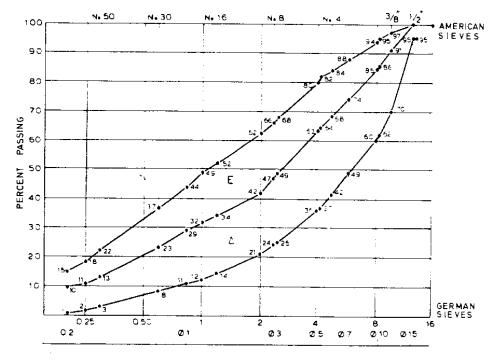
DIAGRAM II : GRADING LIMITS FOR AGGREGATES OF MAXIMUM GRAIN PASSING  $\Phi$  15, or # 16\*, or 1/2"
