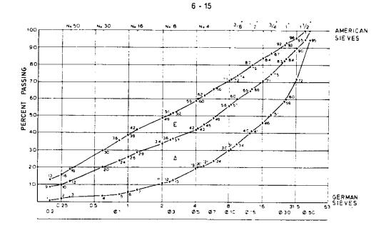
DIAGRAM II : GRADING LIMITS FOR AGGREGATES OF MAXIMUM GRAIN PASSING  $\Phi$  50, or # 63\*, or 1 1/2"
