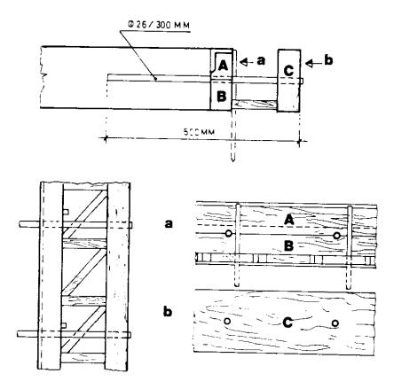
It is recommended that the bars are steeped in thick asphalt solution to provide bond breaking with concrete
